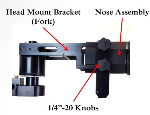
Place a torpedo level on top of the Head Mount Bracket. If not level, use a hex wrench to loosen (2) 3/8"-16 Hex Head Bolts, which are inside the Nose Assembly (see below). Rotate the Nose Assembly until level is achieved. Then tighten these bolts.
