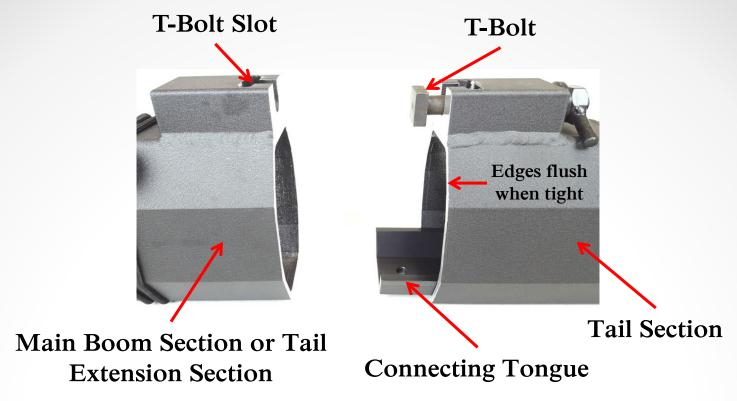
While lowering the T-Bolt from the Tail Section into the T-Bolt Slot on top of the Main or other section, slide the Connecting Tongue from the adjoining Tail or other extension section toward the Main Section, aligning screw holes. Insert the Mounting Knob through the aligned holes in the bottom of the Main Boom Section. Then tighten the Mounting Knob. Repeat this process for remaining Boom Sections.
