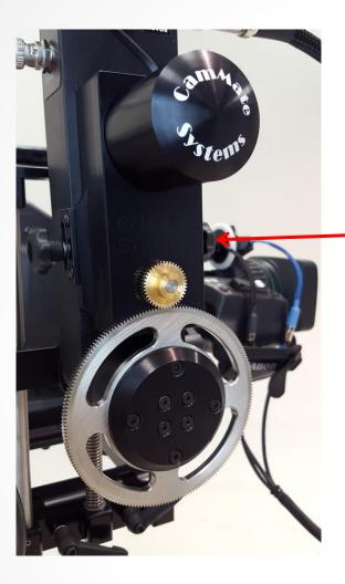
1. Loosen the two Motor Knobs, then slide the Tilt Motor until the gears mesh, and then tighten the Motor Knobs.
