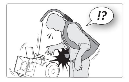
If you fall into water while wearing the Easyrig VARIO 5, it's important to get the equipment off quickly. Just release the waist, chest and shoulder strap buckles. Then slide the shoulder straps over and off of your arms.
