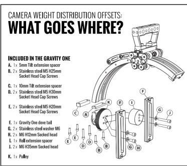
The default configuration of the Gravity One is for camera weights between 6-12 Kg.
