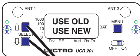
Use the SEL Up and Down arrow buttons to select the old or new frequency.
